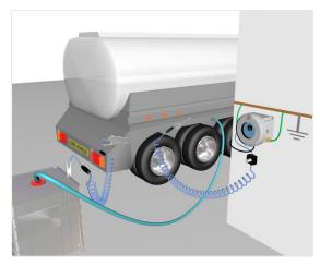
Example of grounded truck bonded to IBC
